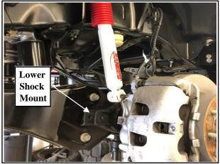
6. Disconnect the end links to the sway bar, frame brake line bracket and **OE** shocks. (both sides).
