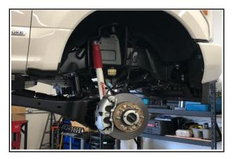
8. Compress spring down, install new coil spacer, poly ring, **OE** spring isolator and reinstall spring. Be sure to line up the previ-ously applied coil spring reference mark.
