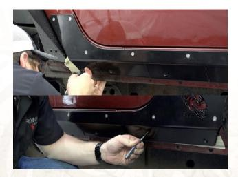
Again, remove the part from the body. Drill all hole locations and install nutserts per steps **4**) and **5**).
