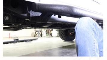
Insert the single M12 bolt and washer into the bottom of the rear most bracket with an 18mm socket. Tighten down each nut and bolt until the slider is tight against the frame.
