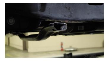
On the passenger side and with an 18mm socket, remove the center gas tank skid plate bolt.
