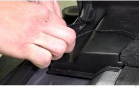
Push the conduit through the rubber seal illustrated in Step #2 and pull it through to the driver's side taillight.
