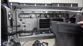
Using a flat head screw driver open the drivers side taillight access panel, remove the plastic bolt using a T-40 Torx Bit. Remove the taillight and disconnect it from its power.
