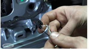
With the long Backside wire, run it through the tailgate wrap, make sure there is an inch or two of slack so the wires are not stressed excessively when the Tailgate opens.
