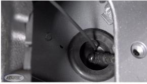
Using a body clip removal tool, pull the OEM license plate light connector and route it through the driver's side light cavity.
