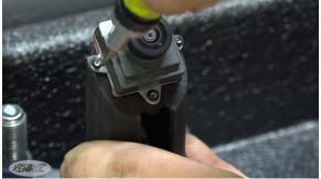
Using a T-6 Torx bit unscrew the Backup camera from its mount. And remove the camera feed cable. Carefully place the camera aside.
