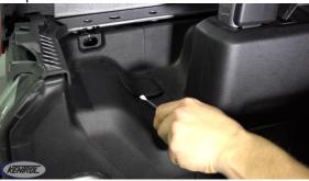
Using a flat head screw driver, pull away the driver's side inner panel enough to fit your arm. \*If you choose to hide your wiring, use a pair of scissors to carefully make a cut into the tailgate fabric cord wrap and push wiring through.
