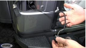
Strip the license plate connector wires and connect to the longer Backside cables: Red to white and black to black. Make sure these connections are properly insulated. Push the wires back into the taillight cavity.
