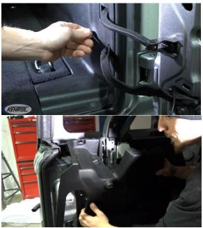
Make a cut into the rubber conduit seal just above the driver side taillight. (NOTE: Wires will be pushed through later)
