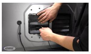
Using a 4mm Allen Wrench and 12mm socket with the included button head bolts secure your license plate to the backside.
